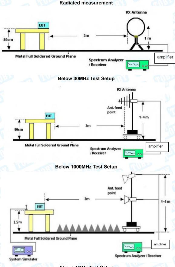
Above 1GHz Test Setup
