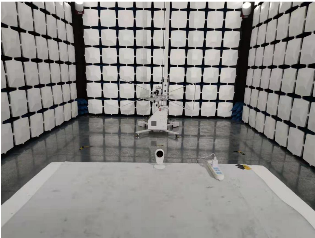
Below 1GHz for radiated emission test setup
