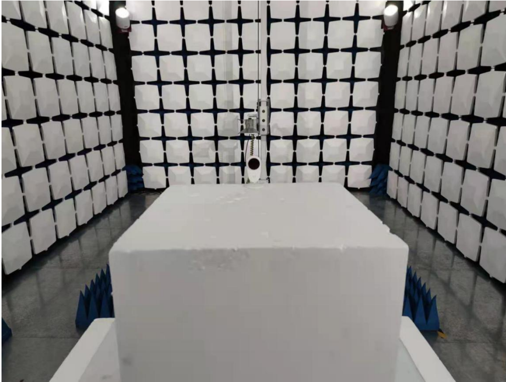
Above 1GHz for radiated emission test setup
