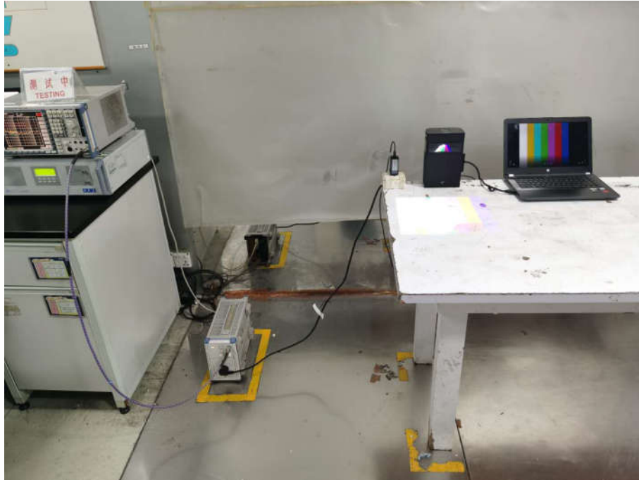
AC Conducted Emissions Test Setup
