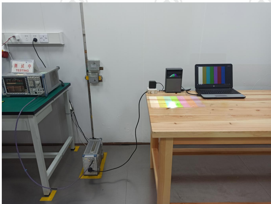
Conducted Emissions Test Setup
