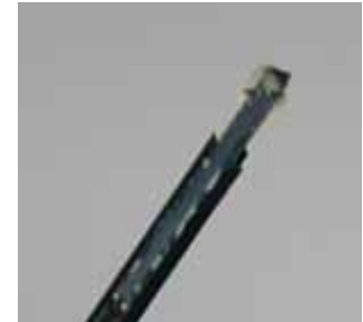
EX3DV4 E-Field Probe
