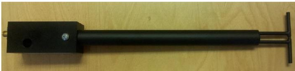
Figure 1 – MVG COMOSAR Validation Dipole
