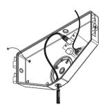
Plug the incoming PoE cable into the Power Supply RJ45 port, labeled PoE. Ensure a good connection.
