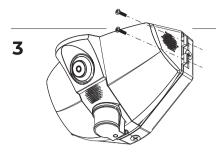
Separate the two halves of the floodlight by losening the two enclosure screws and pivoting the hinge open.
