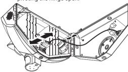
Remove the white Molex connector at the green circuit board, coming from the power supply (depress the tab and gently wiggle the connector to remove) and the green grounding wire.
