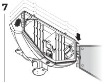
Attach front half of Niō Floodlight to the mounting plate ® by sliding it onto the hinges.
