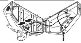
Reconnect white Molex connector and black grounding wire that were disconnected in Step 3. Optionally, use the provided Ethernet Patch Cable to attach the DATA port on the Power Supply to the RJ45 port on the Niō, to supply hard-wired internet via PoE.
