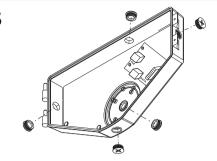
Choose one of the five conduit plugs to remove and connect the electrical conduit through it to supply power to the floodlights. Typically, there will be a ground wire between the housing and the wall that would need to be disconnected and reconnected.
