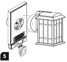
Now that the wiring is connected, mount your light fixture of choice to the CWP following the instructions for your specific light fixture. Install a lightbulb if necessary. (maximum wattage: 60W)
