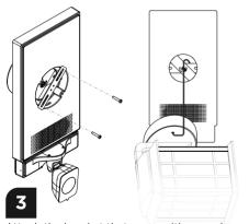
Attach the bracket that came with your chosen light fixture to the CWP by threading the two short screws into the two protruding posts of the CWP bracket. Adjust and level the light fixture bracket as necessary. Now use the provided holding hook (F) to suspend the light from the bracket you just installed, and free your hands for wiring.
