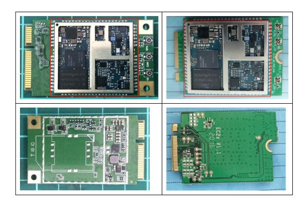
The LTE modular which supports WCDMA/LTE function. For use in the US market, this modular only support WCDMA Band 2/5, LTE band 2/4/5/12/13/66/71, the other WCDMA/LTE bands was disabled by the manufacturer in the software. The end user has no capability to activate it.
