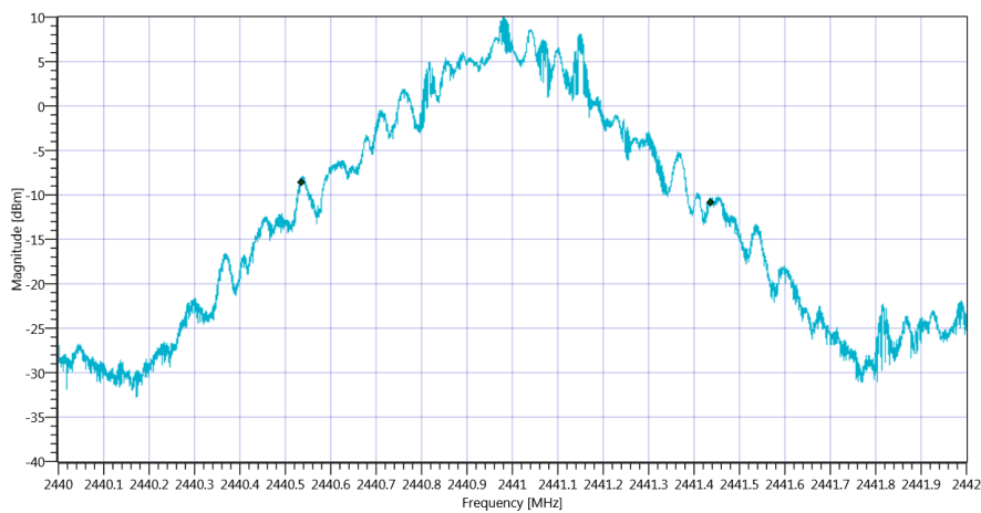
Plot_FCC Part 15.247 Bandwidth 99PCT-20dB ~ BT Classic Basic rate 99PCT_06072020_144414.png
