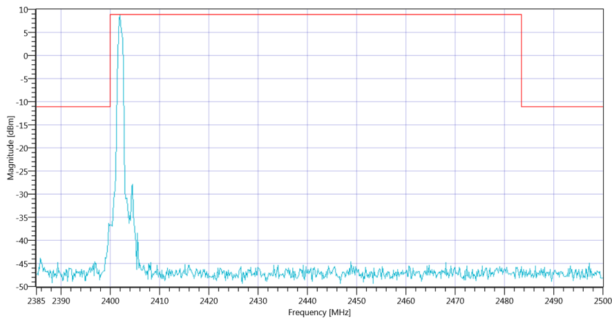
Plot_FCC Part 15.247 TX Spurious Conducted ~ BT Classic EDR 8DPSK 2402_06072020_154244.png
