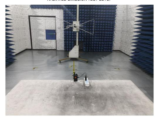
RADIATED EMISSION ABOVE 1G TEST SETUP
