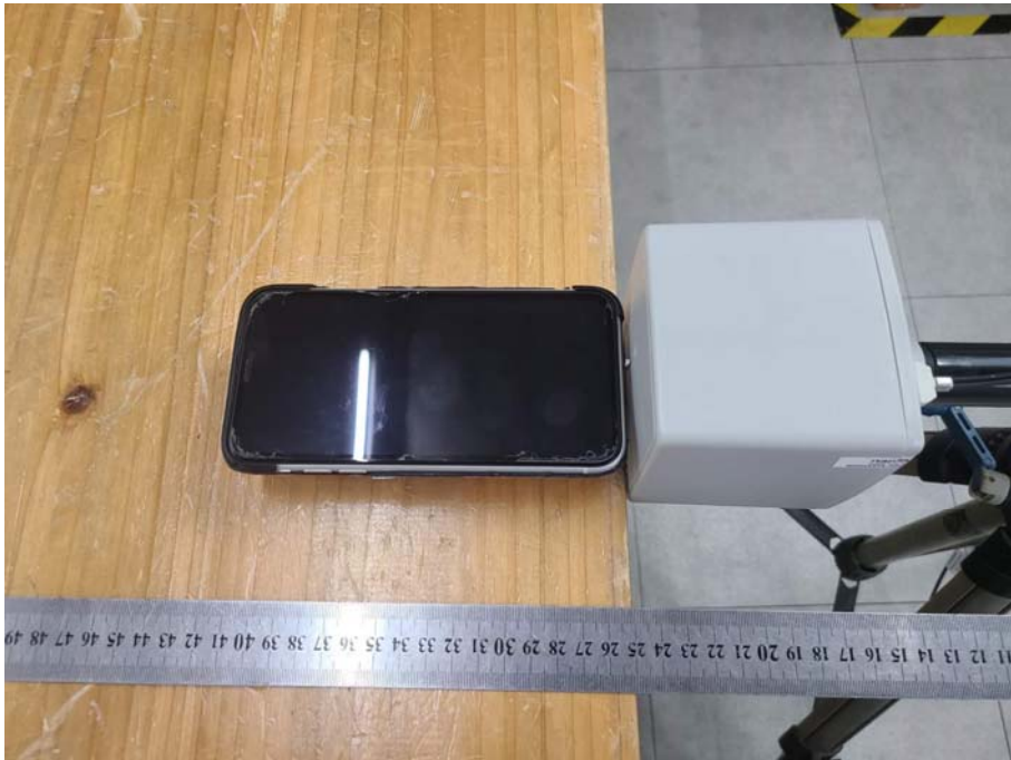
Test Position C-0cm from the edge of EUT to the geometric center of the probe
