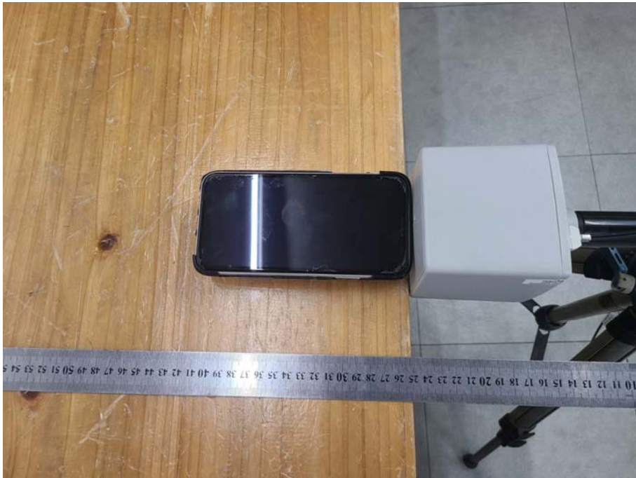
Test Position A-0cm from the edge of EUT to the geometric center of the probe
