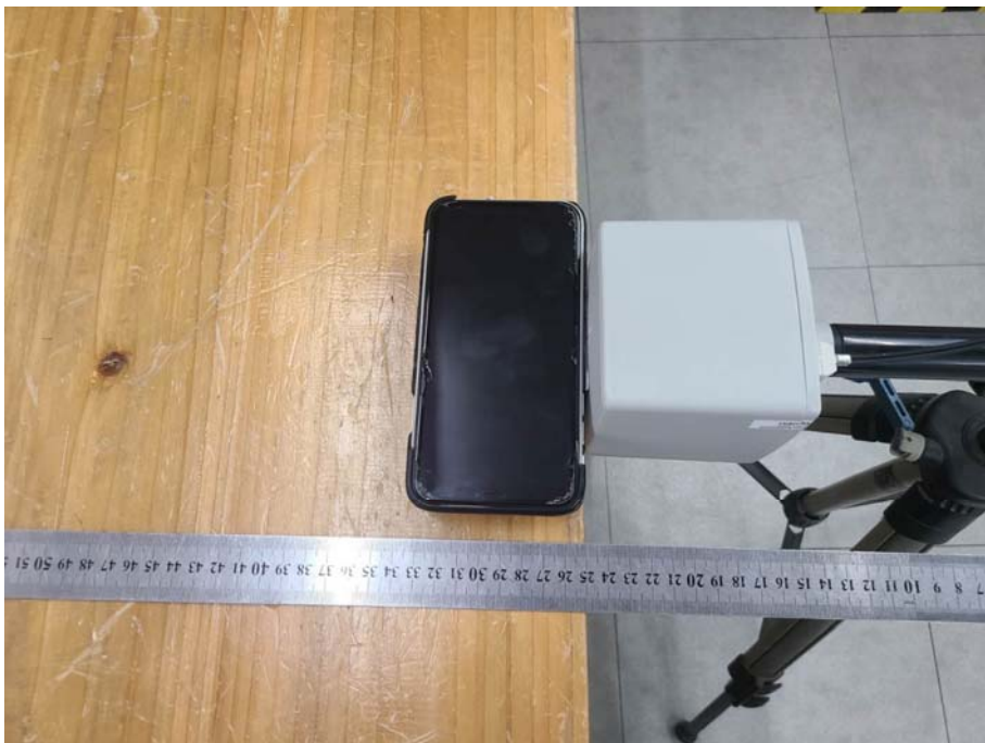
Test Position B-0cm from the edge of EUT to the geometric center of the probe
