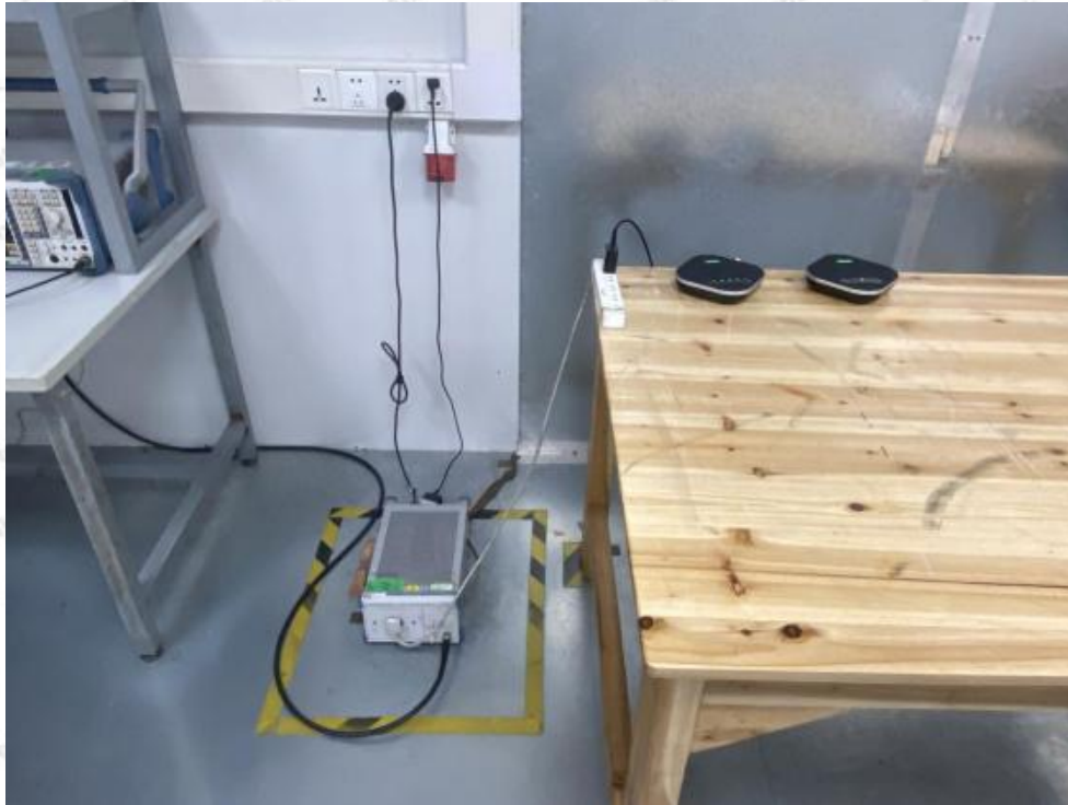
Photo of Conducted Emission Measurement
