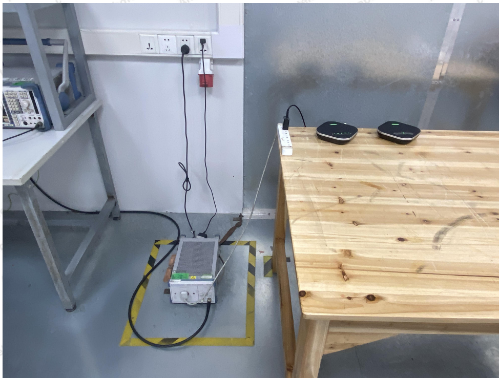
Photo of Conducted Emission Measurement
