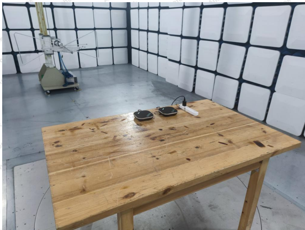
Photo of Radiation Emission Test
