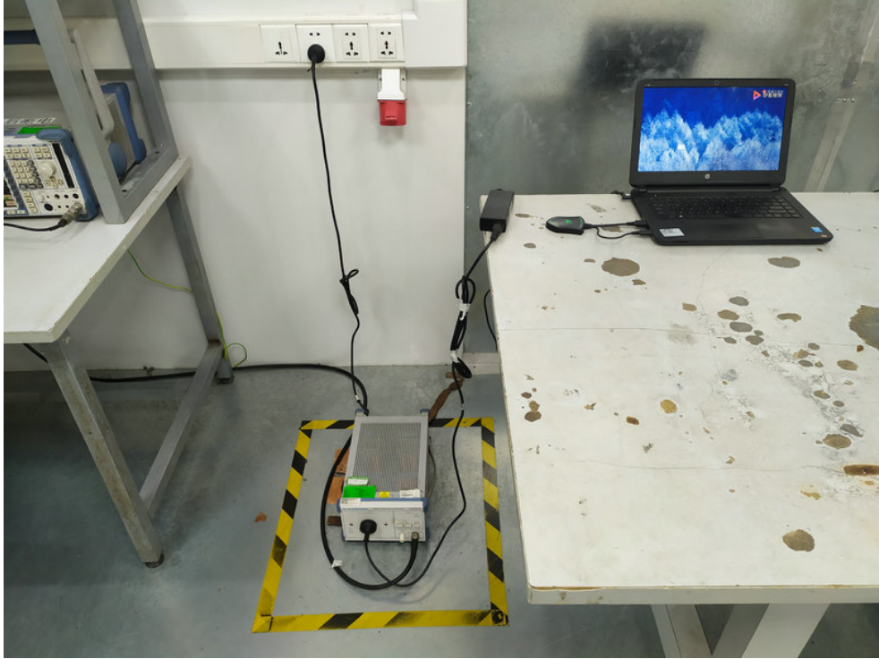
Photo of Power Line Conducted Emission Test
