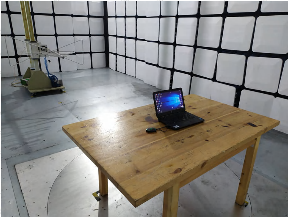
Photo of Radiation Emission Test
