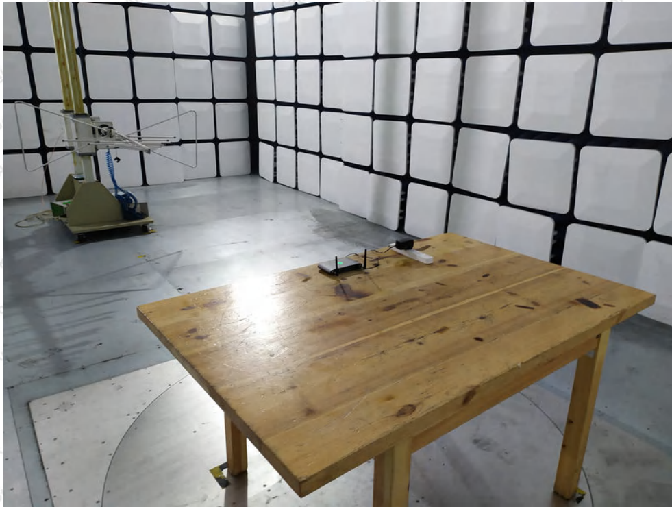
Photo of Radiation Emission Test
