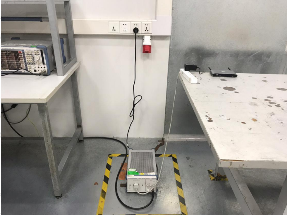
Photo of Power Line Conducted Emission Test
