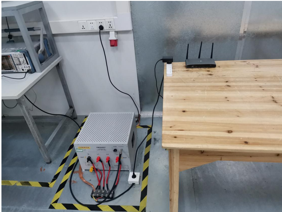
Photo of Power Line Conducted Emission Test
