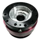
After opening the quick release second lock, To remove the quick release, press the button to remove it
