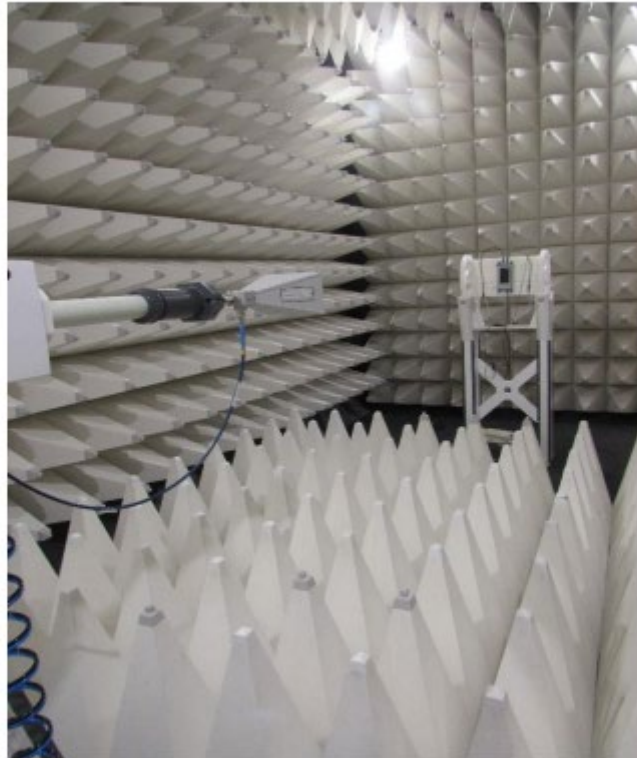
Setup for measurements above 1 GHz
