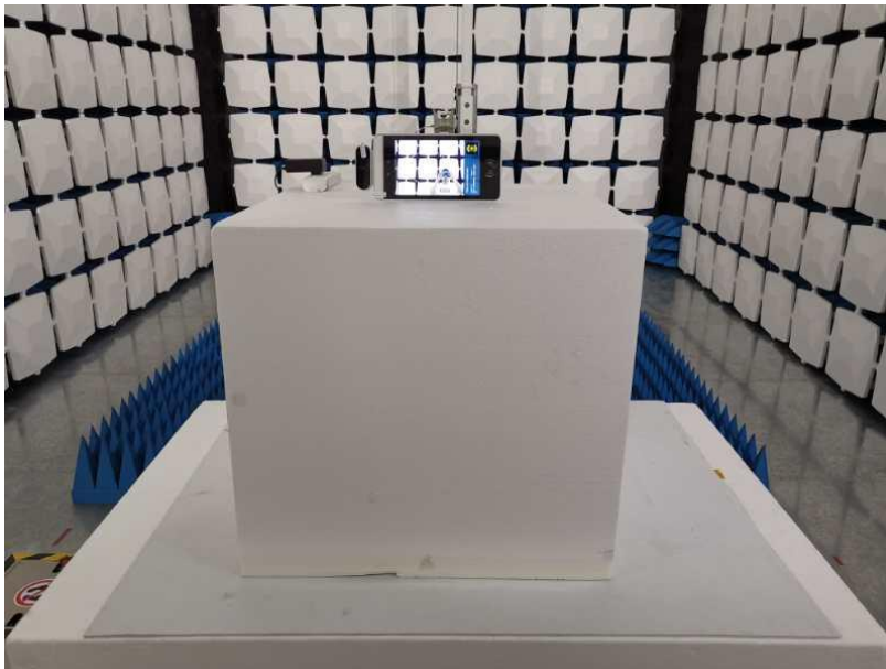
Conducted Emission test setup
