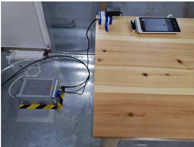
Conducted Emission test setup
