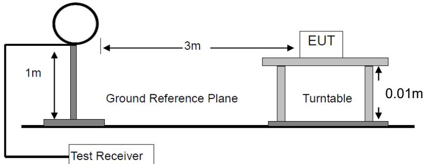
For Radiated Emission 30-1000MHz
