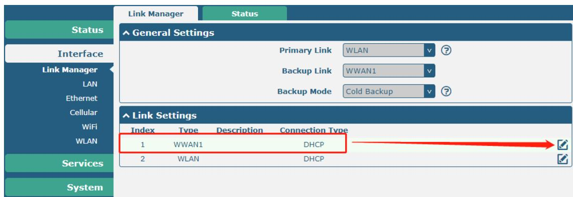
Configure APN in WWAN Settings, select "Automatic APN Selection" as OFF; you can manually configure APN, authentication method, user name and password, etc.;
