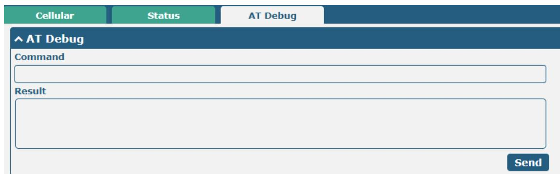
The screenshot shows a user interface for AT Debug. At the top, there are three tabs: 'Cellular' (highlighted in green), 'Status' (highlighted in blue), and 'AT Debug' (highlighted in white). Below the tabs is a section titled 'AT Debug' with a small upward arrow icon. This section contains two text input fields: 'Command' (labeled 'Command') and 'Result' (labeled 'Result'). At the bottom right of this section is a blue 'Send' button.
