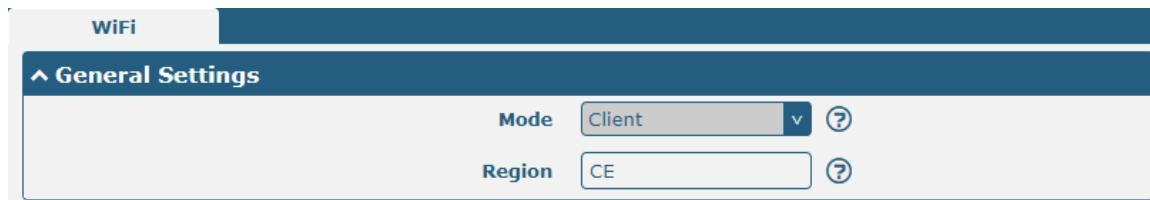
Click "Interface> Link Manager> Link Settings" and click the WLAN edit button to configure the parameters of the WiFi client in the pop-up "WLAN Settings" window. There can be three configurations, namely the APP Hotspot for the mobile phone APP to set the wifi/Primary Hotspot/Secondly Hotspot.
