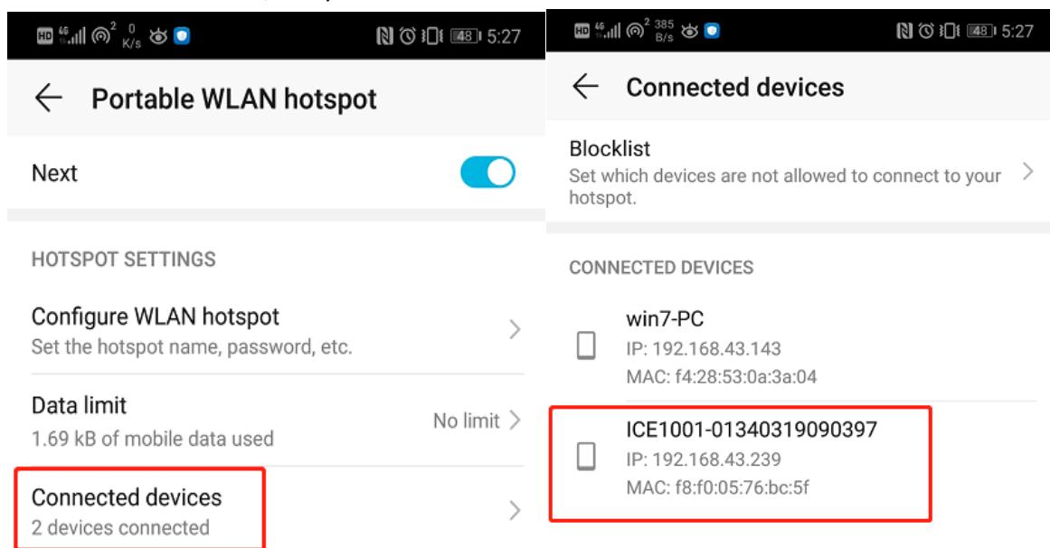
At this point, we can log in to the parameter configuration page of the router through a PC connected to the hotspot, and enter the IP of the router on the browser to log in:
