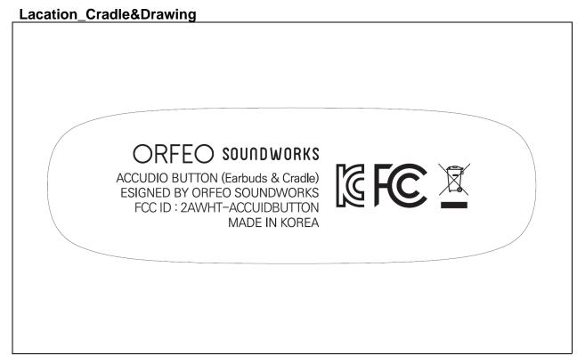
The location of the label is on the Bottom of the Cradle case.
