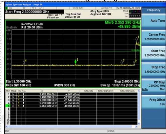
Left Band edge hopping on
