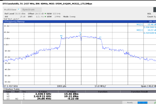
Figure 8.5-4: Minimum 6 dB bandwidth, IEEE 802.11n HT40 (CDD mode), minimum measured DTS bandwidth
