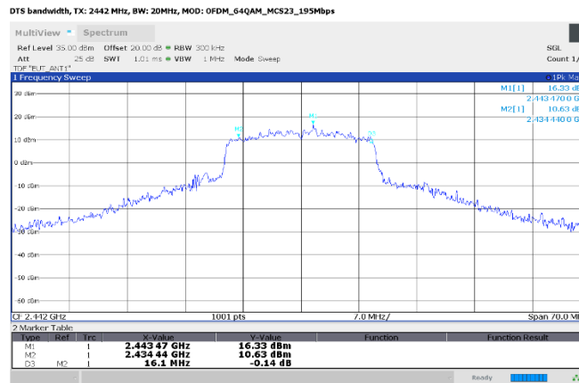
Figure 8.5-3: Minimum 6 dB bandwidth, IEEE 802.11n HT20 (CDD mode), minimum measured DTS bandwidth
