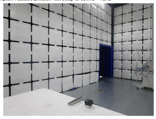
Description: Radiated Emission Test Setup for 1GHz ~ 25GHz
