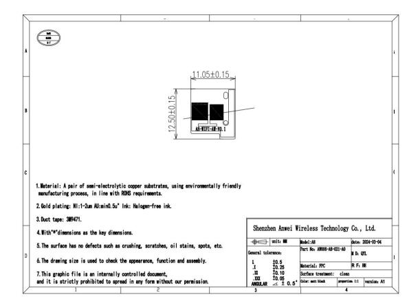
(Working frequency band of 2.4G/5GWIFI antenna): 2400~2500/5100~5800
