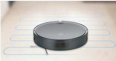
Automatic Cleaning Mode Cleaning Path
