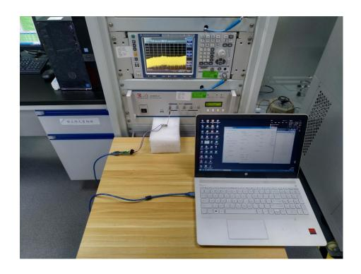
Conducted Emission For AC Mains Power Ports (Adapter 1)
