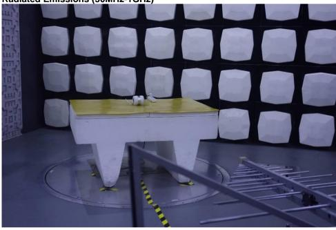
Radiated Emissions (9kHz-30MHz)
