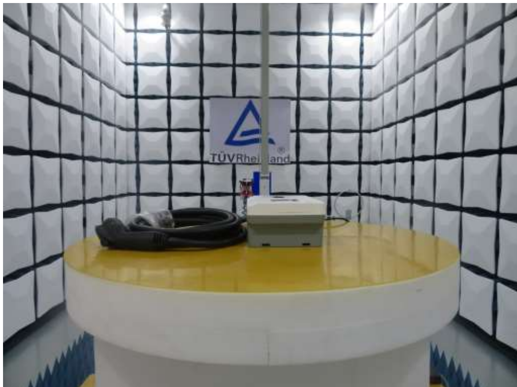
Photograph 2: Set-up for Radiated Spurious Emission, Above 1G
