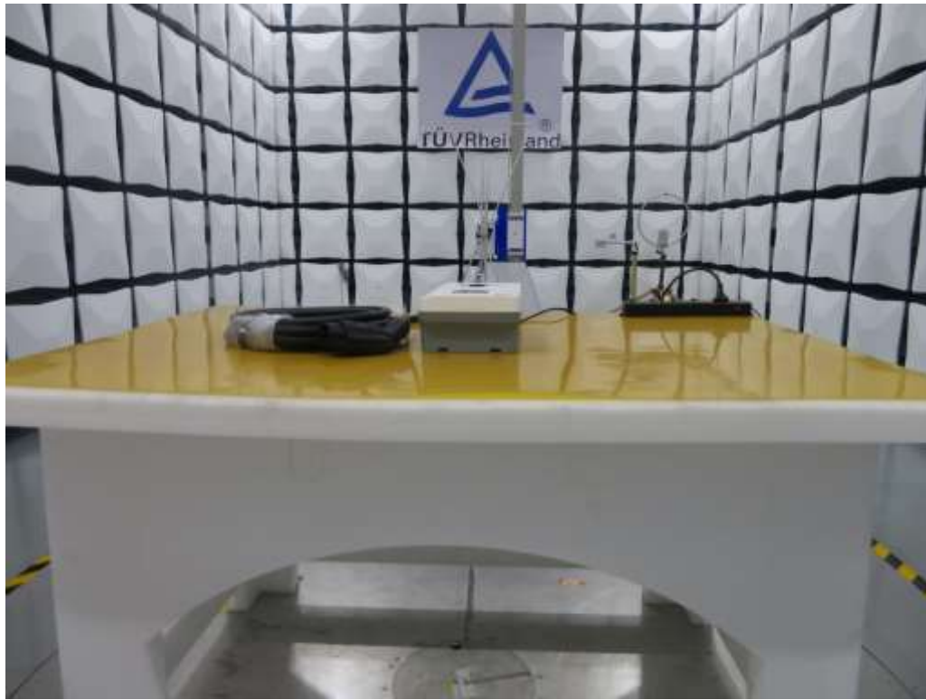
Photograph 1: Set-up for Radiated Spurious Emission, 30MHz - 1GHz
