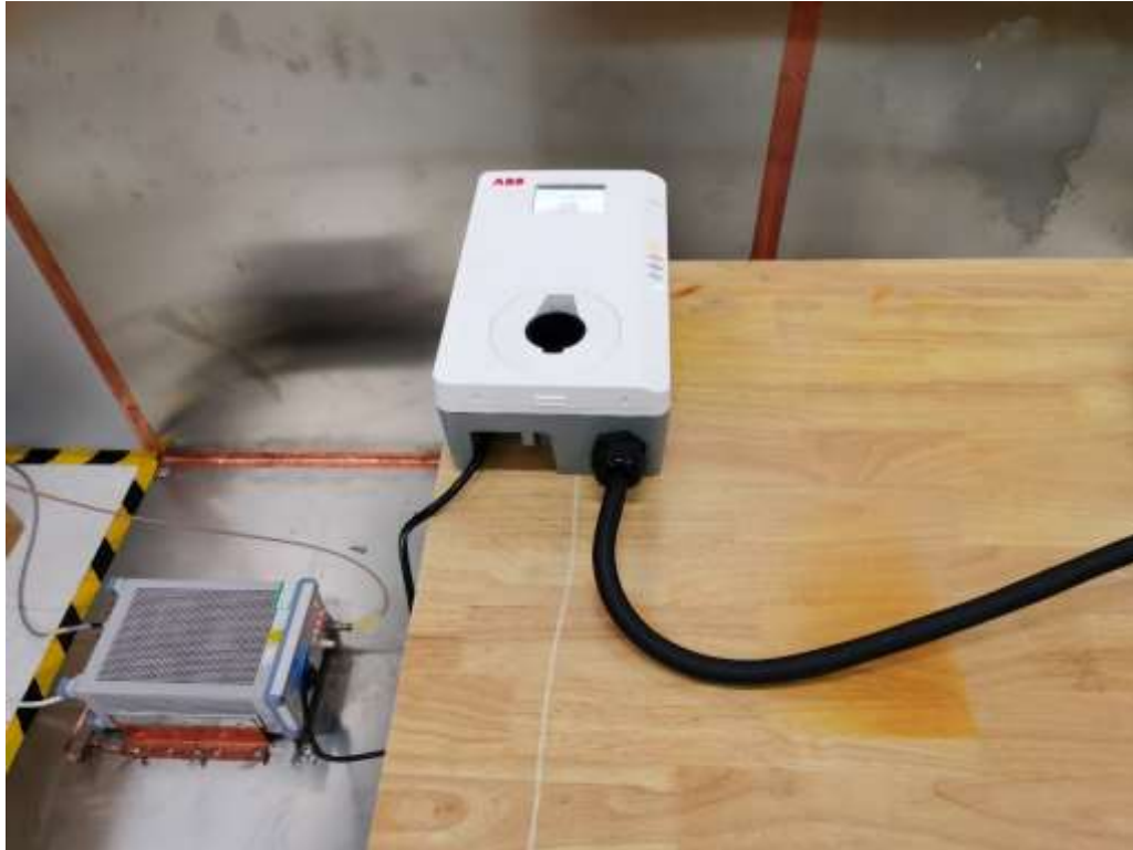
Photograph 3: Set-up for Conducted Emission
