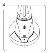
An indicator will illuminate BLUE on the Power Dock when connection is established. The Peak Pro will also illuminate and pulse while charging. \*Tip - Align Peak Pro charging port towards area indicated with arrow for faster charge.
