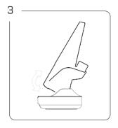
Tilt the Peak Pro forward into the Power Dock and then push down into the base to begin wireless charging.
