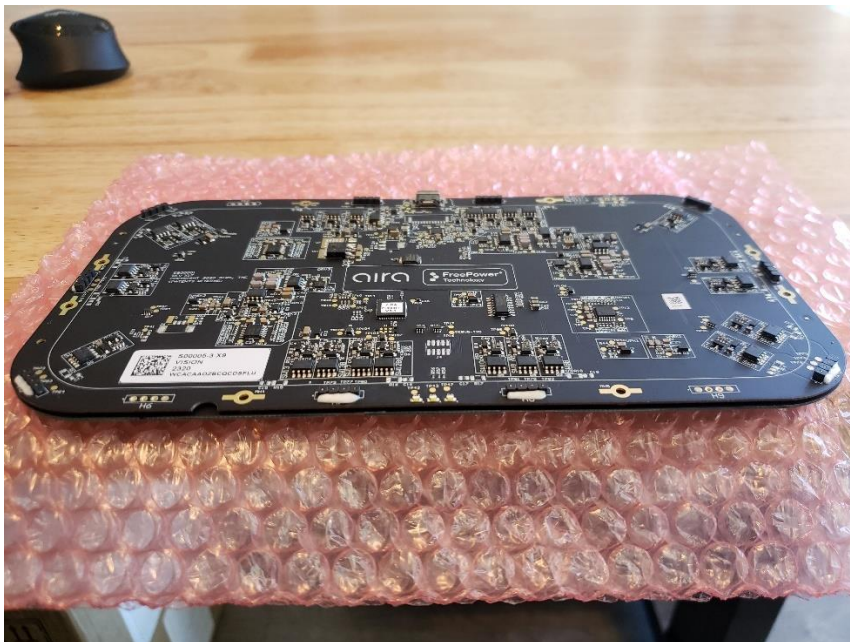
Component side – LED's sides
