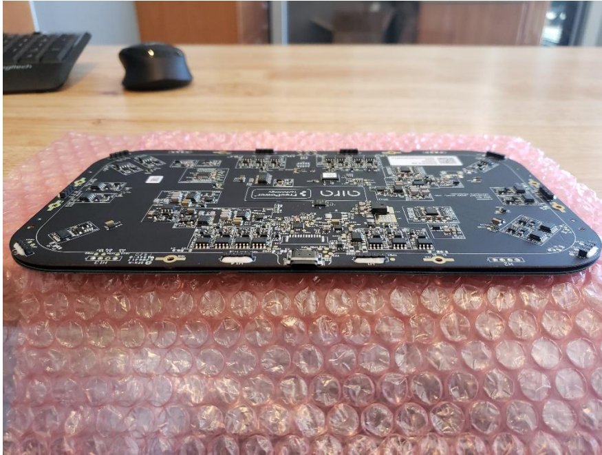
Component side – USB C connector
