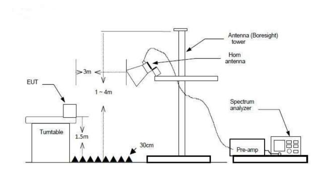
Figure 5. Radiated Emission Above 1GHz Test Setup
