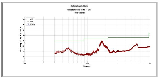
Plot 1 – Radiated Emissions – 30MHz to 1GHz
