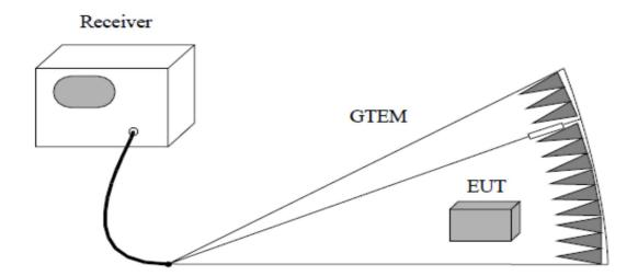
Figure 1. Radiated Emissions Test Setup (30MHz – 1GHz)
