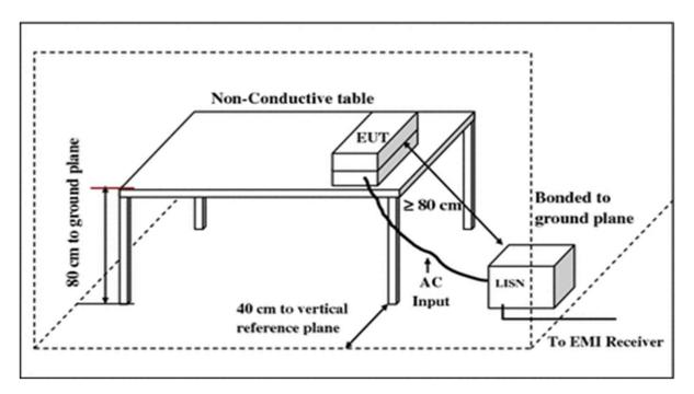
Figure 2. Conducted Emissions Test Setup
