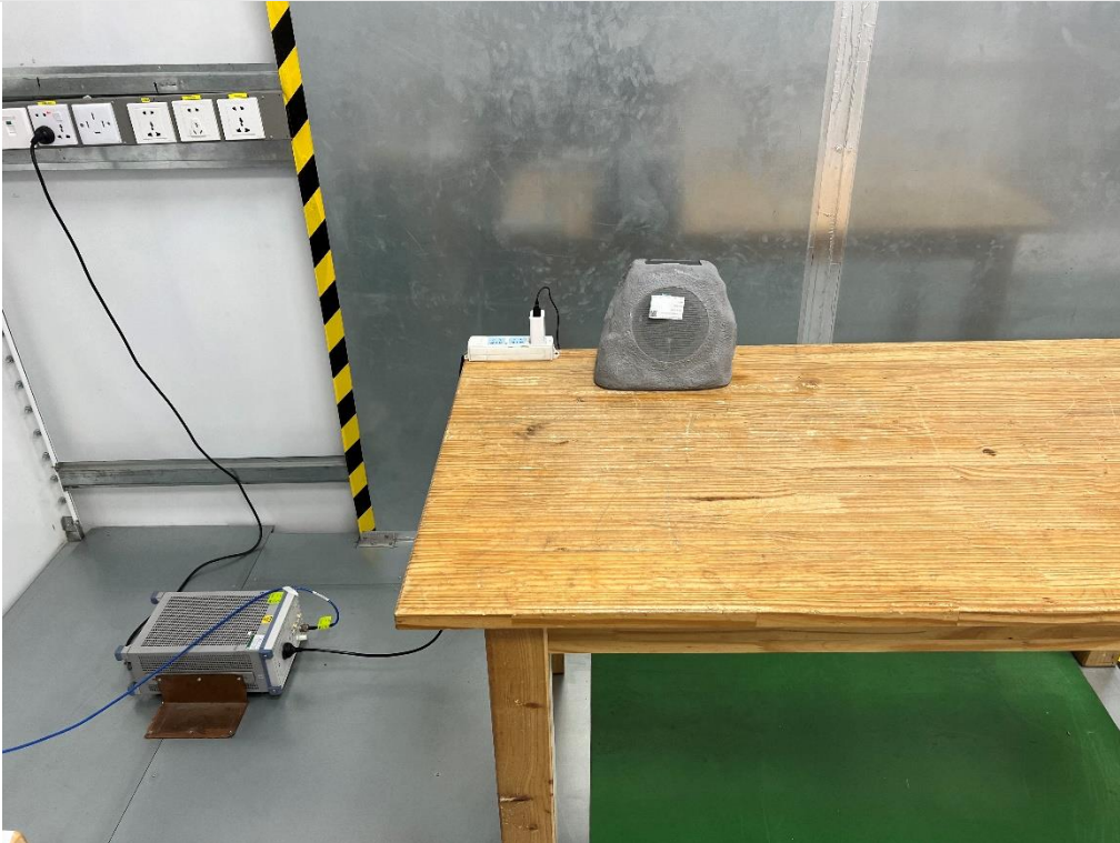
AC Power Line Conducted Emission
