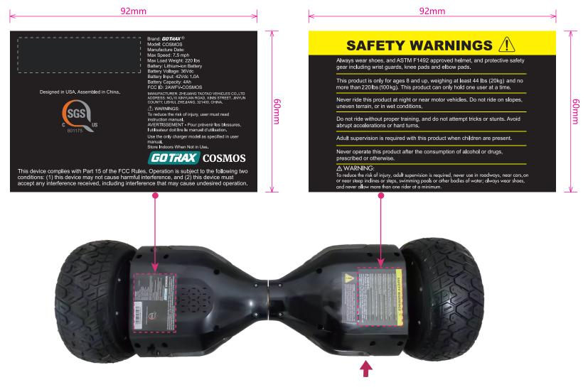
The label is attached to the bottom plate.
