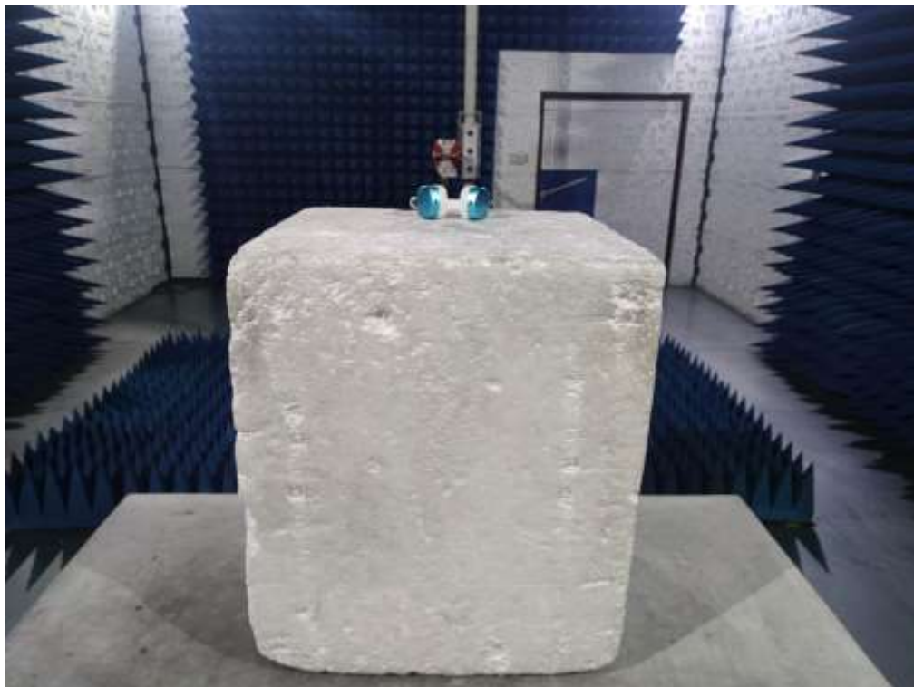
RADIATED EMISSION TEST SETUP ABOVE 1GHz
