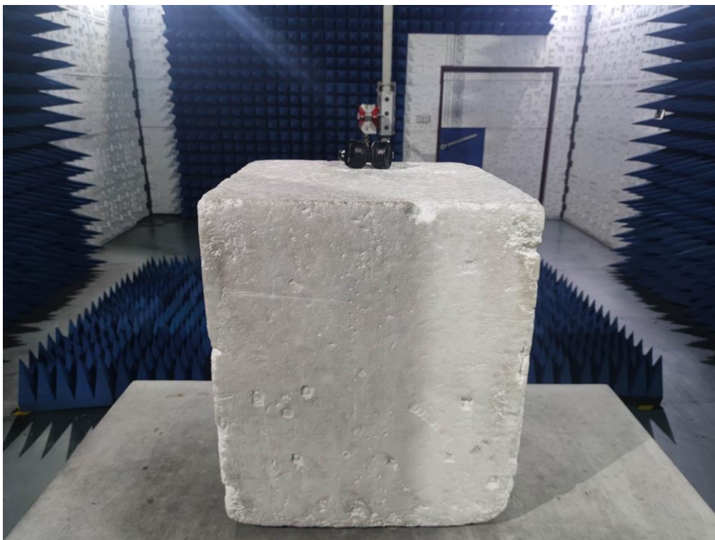
RADIATED EMISSION TEST SETUP ABOVE 1GHz
