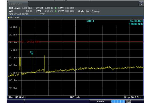
Test mode : Bluetooth LE / Lowest Frequency\_Conducted Spurious Emission
