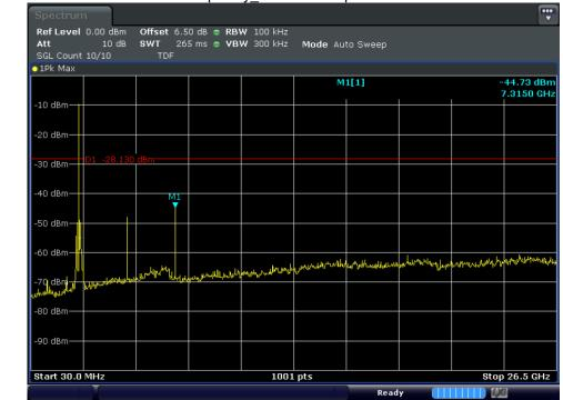
Test mode : Bluetooth LE / Middle Frequency\_Conducted Spurious Emission
