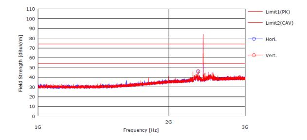
Test mode : 1 GHz ~ 3 GHz\_( Worst case : Bluetooth LE / Lowest Frequency )
