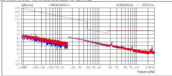
Test mode: 30 MHz ~ 1 GHz (Worst case: 2 402 MHz)
