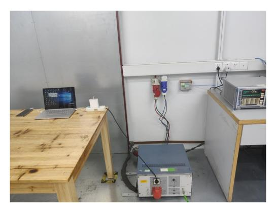
FCC RADIATED EMISSION TEST SETUP
