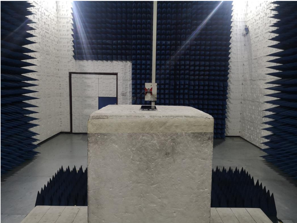
RADIATED EMISSION TEST SETUP ABOVE 1GHZ
