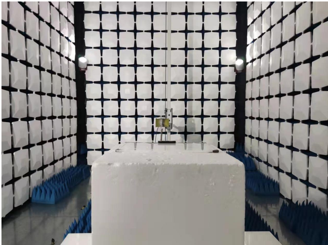
Above 1GHz for radiated emission test setup
