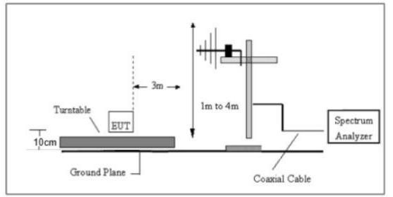
(C) Radiated Emission Test-Up Frequency Above 1GHz
