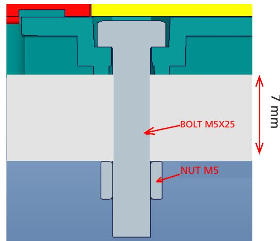
You have to remove the nut before mounting the FS3 on the bed and after mounting the FS3 to the bed, the nut is fastened to secure that the FS3 is fixed to the bed frame.
