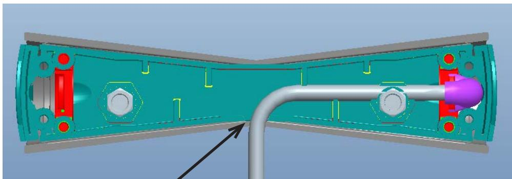
Location of the notch for the cable of the FS3 bed model.
