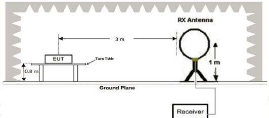
2. Radiated Emission Test-Up Frequency 30MHz~1GHz
