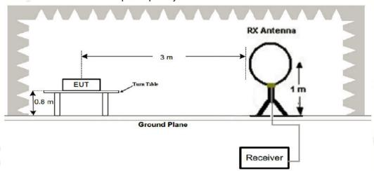
2. Radiated Emission Test-Up Frequency 30MHz~1GHz
