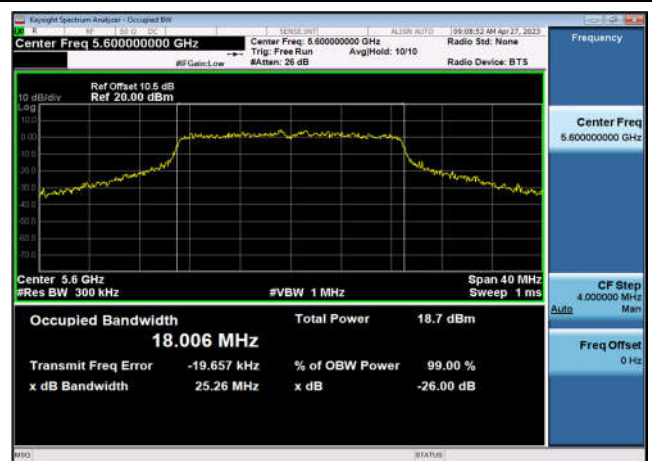
U-NII-2c 26dB&99% Bandwidth-802.11n(20MHz),5600MHz,Ant1
