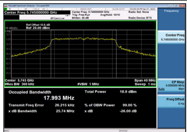
U-NII-3 26dB&99% Bandwidth-802.11ac(20MHz) ,5745MHz,Ant1
