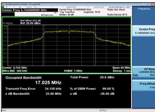
U-NII-3 26dB&99% Bandwidth-802.11a(20MHz) ,5825MHz,Ant1
