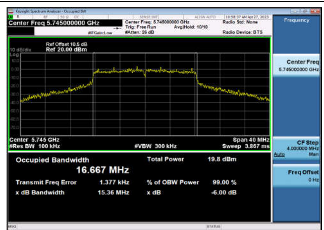
U-NII-3 6dB Bandwidth-802.11a(20MHz) ,5745MHz,Ant1
