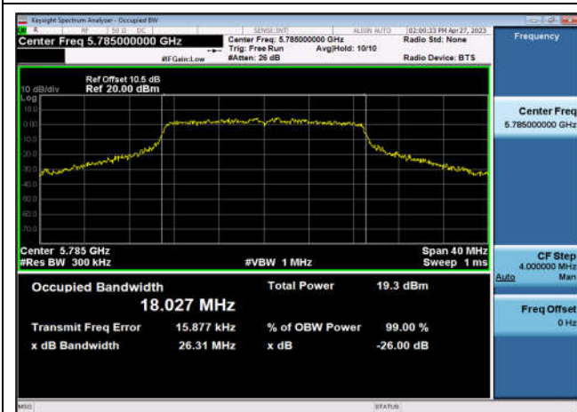
U-NII-3 26dB&99% Bandwidth-802.11n(20MHz),5785MHz,Ant1
