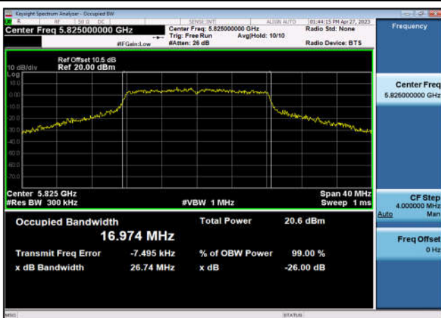
U-NII-3 26dB&99% Bandwidth-802.11a(20MHz) ,5825MHz,Ant1
