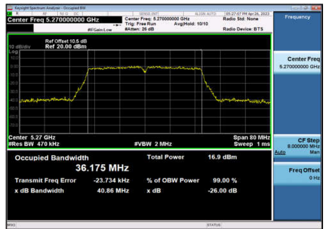
U-NII-2a 26dB&99% Bandwidth-802.11ac(80MHz),5290MHz,Ant1
