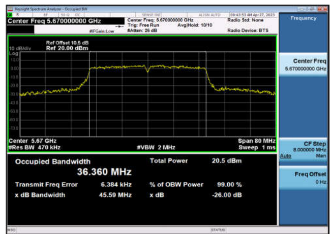
U-NII-2c 26dB&99% Bandwidth-802.11a(20MHz) ,5600MHz,Ant1
