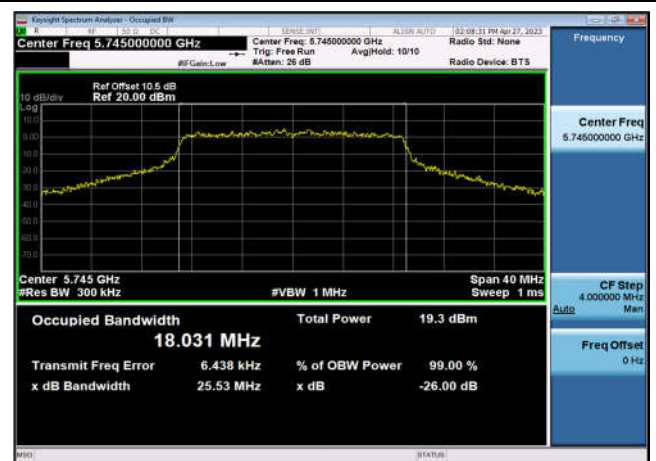
U-NII-3 26dB&99% Bandwidth-802.11n(20MHz),5825MHz,Ant1
