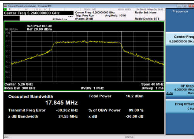
U-NII-2a 26dB&99% Bandwidth-802.11ac(20MHz) ,5260MHz,Ant1
