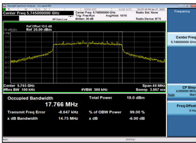
U-NII-3 6dB Bandwidth-802.11n(20MHz) ,5825MHz,Ant1
