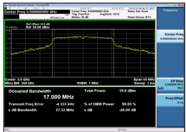
U-NII-2c 26dB&99% Bandwidth-802.11a(20MHz) ,5600MHz,Ant1
