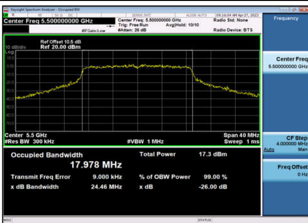
U-NII-2c 26dB&99% Bandwidth-802.11n(20MHz),5500MHz,Ant1
