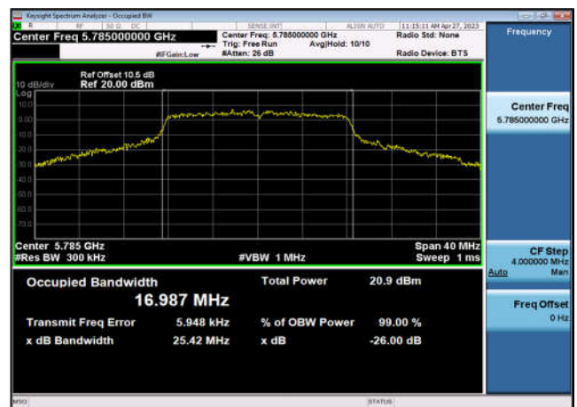
U-NII-3 26dB&99% Bandwidth-802.11ac(20MHz) ,5745MHz,Ant1
